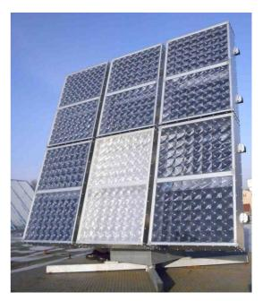
The Fresnel lens array is manufactured by SOG (Silicon on Glass) technology which ensures its low cost and long lifetime. The solar cells with the Fresnel lenses are optimized for maximal power and efficiency.
